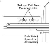
Note: Front location holes are shown. Corresponding rear holes will also need to be marked.
